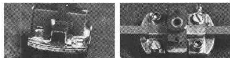
9. Replace the two bottom Mura plates with Certus Super Proofers, and don't use the spacer on the spring post.
