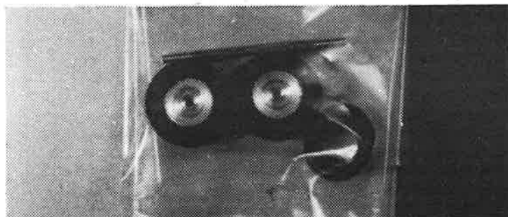
THE STOCK Tyco tires bounce, chatter, and don't bite too well. Replace them with A.J.'s new sponge tires, O-ring fronts, and axles.
