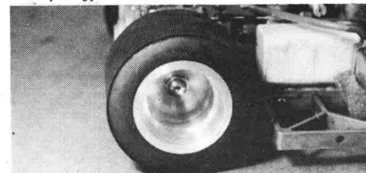
THE GLEAMING Dynamic wheels are twice the width of any other R/C wheel on the market today. They are perfectly scaled - 15" diameter and 18" width. They come in two softness compounds.
