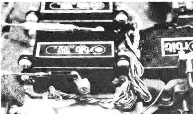
CLOSEUP of a servo. The motor inside activates, through gears, the arm on the outside of the box. The arm is attached to a rod that links it, in this case, to the torque converter. The arm moves back and forth in direct proportion to the command given it by the driver's stick on the transmitter.
