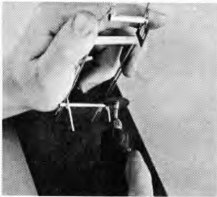
STEP 39 Trim off all of the excess garbage making sure not to wipe out the axle tubes and the other work you and your buddy have labored so long to complete. Trim the main rails at the pencil marks you made earlier.
