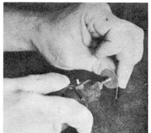
STEP 8 Take your .063 piano wire and cut six pegs each 1-1/2" long.
