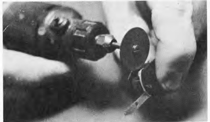
STEP 25 There are a couple extra tabs on your endbell so go ahead and trim away anything not needed.
