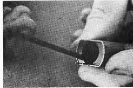
STEP 20 Slip the magnets in the can without the shims for now.
