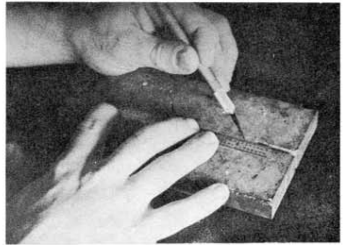
STEP 6 Scribe the centerline through the points you've already marked in Step No. 5. Use your straight edge, it's easier that way.
